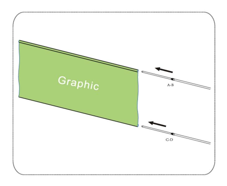
Step 3: Run poles #A-B and #C-D through the pole pockets on the top and bottom of the graphic.
