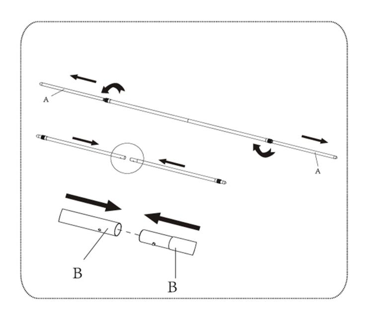
Step 1: Connect the two poles labeled #A-B by joining the B-B ends. Repeat with bottom poles #C-D. Extend telescopic ends A.
