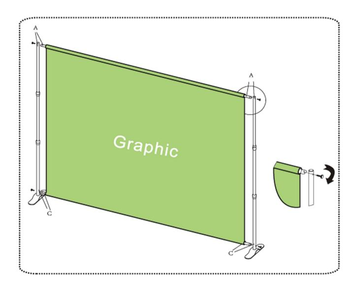
Step 4: Use the black handled thumb screws to secure the horizontal poles to the vertical poles.
