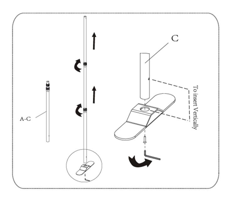
Step 2: Take vertical pole #A-C and insert end C into the pole socket in the base. From the bottom of the base thread hexbolt into end C and tighten.
